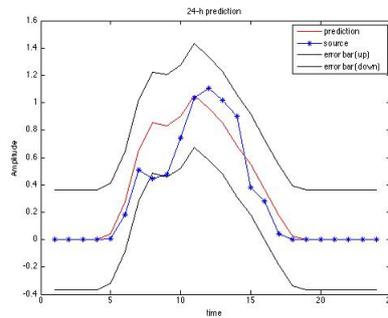
**Fig. 3.** 24-hour PV prediction obtained by MLP NN and Bayesian framework.
