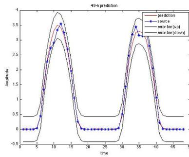
**Fig. 4.** 48-hour PV prediction obtained by MLP NN and Bayesian framework.
