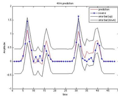
**Fig. 5.** 48-hour PV prediction obtained by MLP NN and Bayesian framework.
