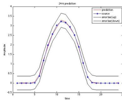
**Fig. 2.** 24-hour PV prediction obtained by MLP NN and Bayesian framework.
