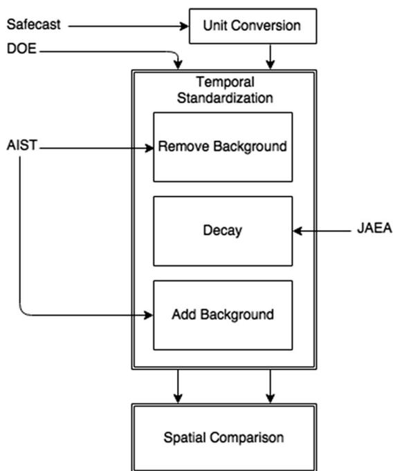
**Fig. 1** Flowchart of the methodology developed to compare Safecast and DOE data which takes into account the spatial distribution of the natural background radiation and of the cesium deposition measured by field surveys
