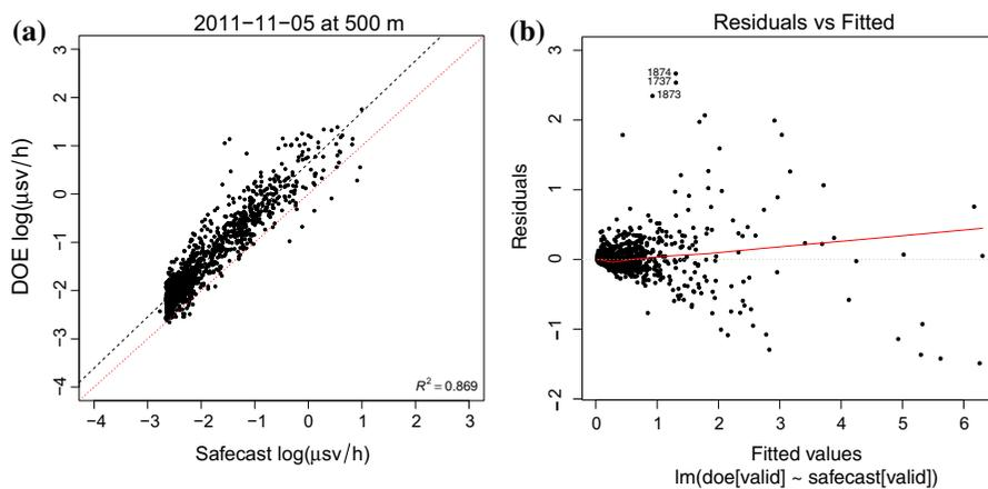
**Fig. 4** Linear model of 500 m<sup>2</sup> at 5 November 2011. **a** Linear model. **b** Residuals of the linear model
