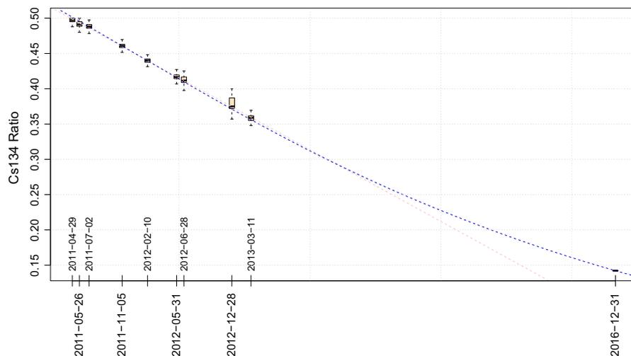
**Fig. 2** Boxplot of distribution of  $^{134}\text{Cs}/^{137}\text{Cs}$  ratio at each survey date with outliers
