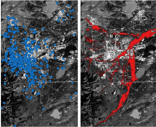
Fig. 2. Flood data set. (Left) Panchromatic image of the city of Boulder, CO, USA, taken on September 17, 2013 from Landsat 8 satellite image, overlaid with geolocated tweets. (Right) UFE as our ground truth.
