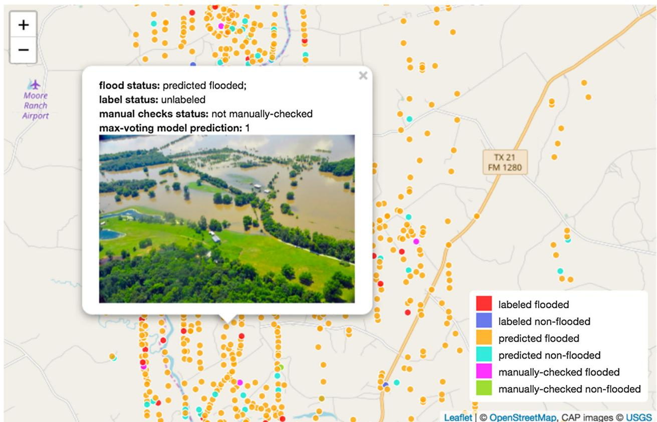
**Fig. 8** A zoomed-in detail for Fig. 7. The value of max-voting model prediction for the demonstration aerial image (i.e., 1) means the trained max-voting model automatically classifies this aerial image as flooded
